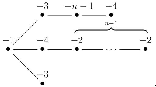
When  $n = 1$  we get  $\Sigma(2, 5, 17)$  and  $\Sigma(3, 4, 17)$ . Surgery diagrams for their canonical negative definite plumbings appear as the gray components in Figure 2 and Figure 3, and the black component gives the necessary surgery to  $Y$ . This can be seen from a straightforward sequence of blowdowns which we leave to the reader.
